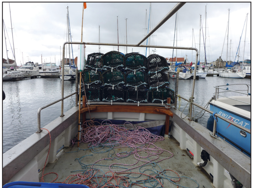
Figure 2: Illustration of the potential hazard associated with loose ropes on deck
